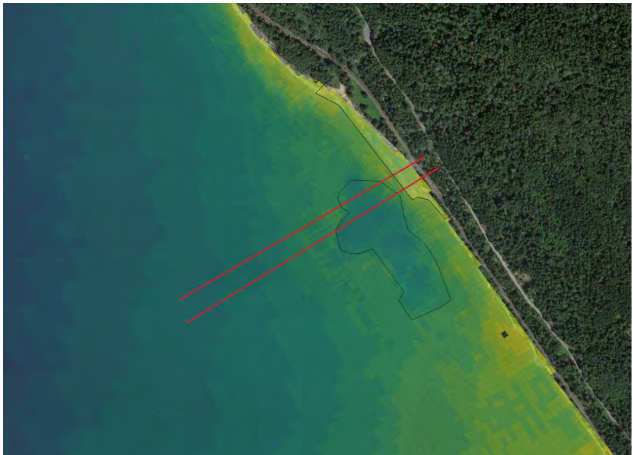
Figure A-4. Existing surface, dredged area included (model label “Dredged”), at low tide. Note that the model extends well over the beach.
