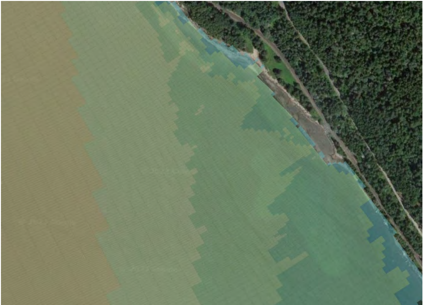
Figure 28. Significant Wave Height at 3.28 Average Wave Height, Restored and Filled Surface (model label "Alt_Filled").
