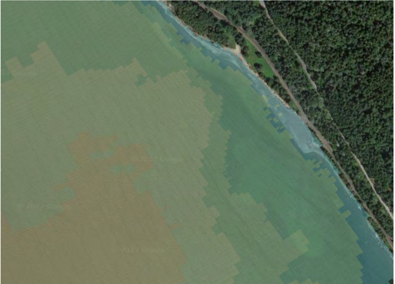
Figure 27. Significant Wave Heights at 0.33 Feet Average Wave Height, Existing Conditions (model label "Dredged").
