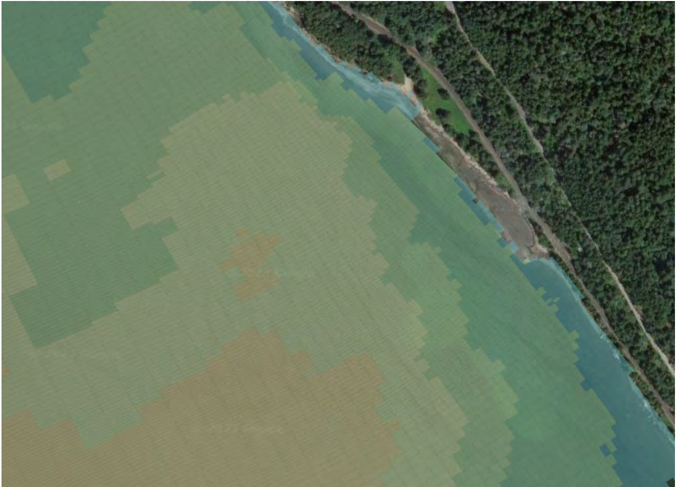
Figure A-21. Significant wave height at 0.33 average wave height, restored and filled conditions (model label "Alt_Filled"). High significant wave heights have been shifted offshore.
