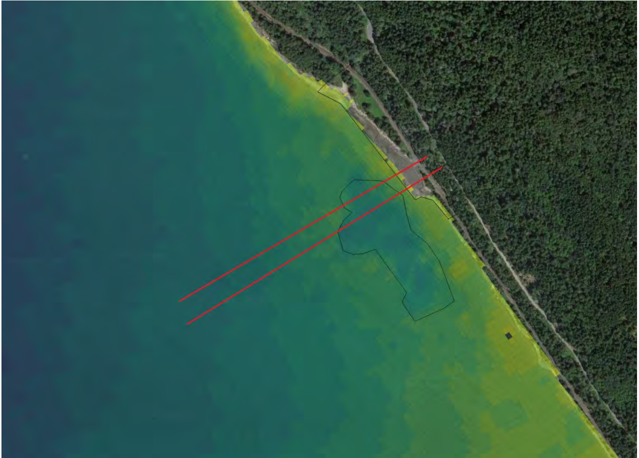
Figure A-5. Alternative restored surface, dredged area included (model label "Alt_Dredged"), at low tide. Note that in the restored surface the model edge is pushed seaward, reflecting a raised and nourished beach.
