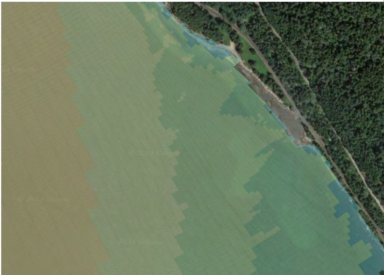
Figure A-22. Significant wave height at 3.28 average wave height, restored and filled surface (model label "Alt2_Filled"). The restored beach buffers the high waves away from infrastructure.
