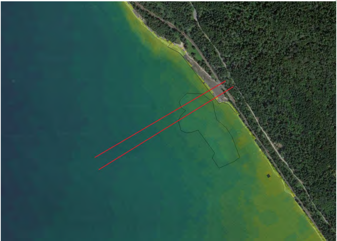
Figure A-7. Alternative restored surface, dredged area filled (model label "Alt_Filled"). Note that in the restored surface the model edge is pushed seaward, reflecting a raised and nourished beach.
