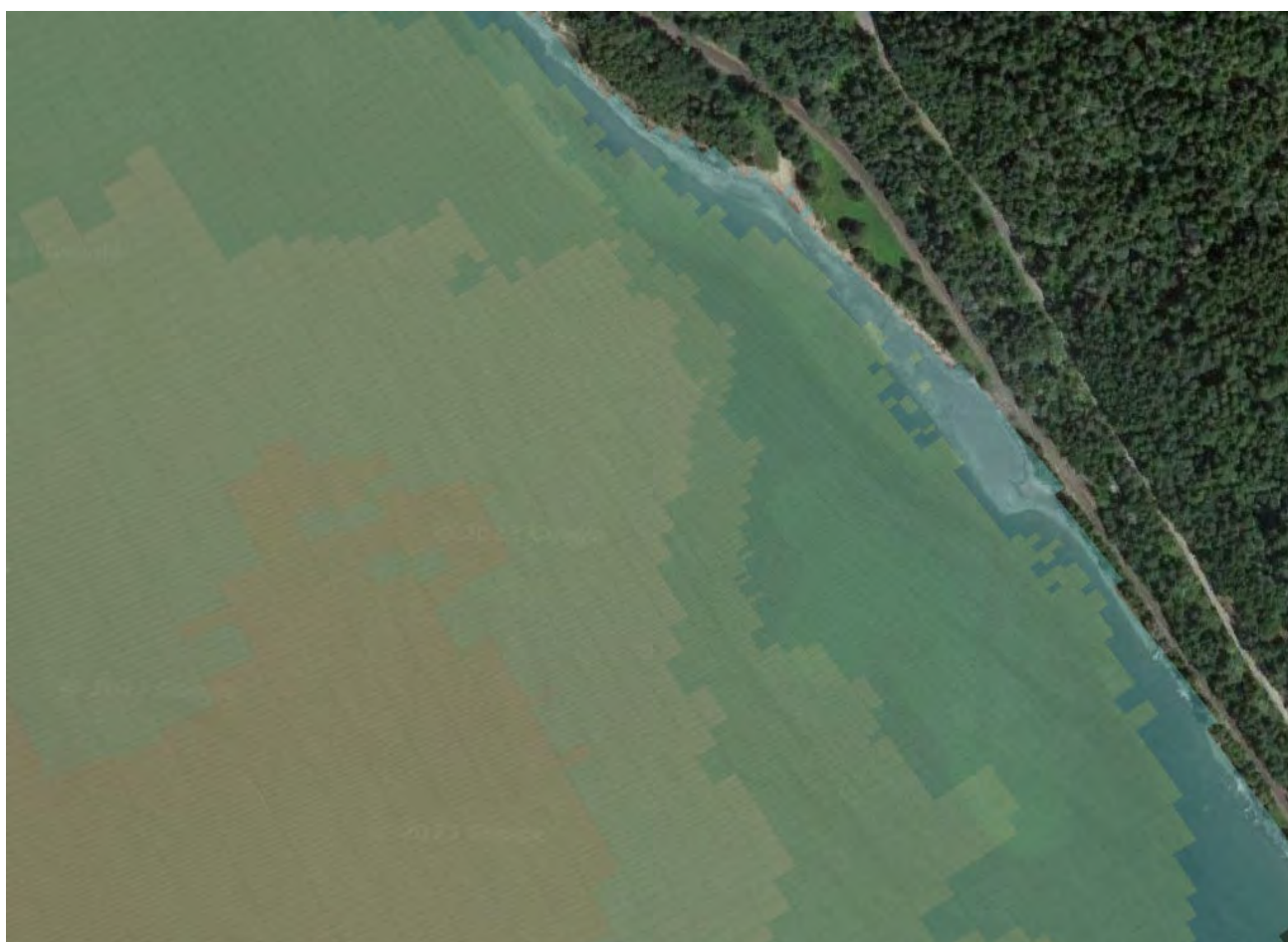
Figure A-19. Significant wave heights at 0.33 feet average wave height, existing conditions (model label “Dredged”). Note the encroachment of higher waves on Clayton Beach.
