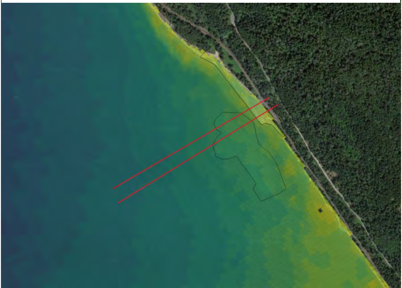
Figure A-6. Existing surface, dredged area filled (model label "Filled"), at low tide. The dredged area no longer displays the deeper bathymetry present in Figures A-4 and A-5. Note that the model extends well over the beach.
